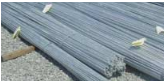
Straight lengths of galvanized rebar
